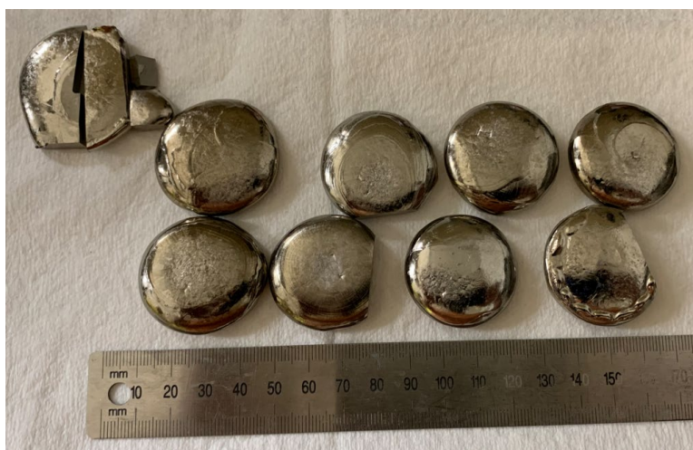
Figure 1: Arc melted U-50Zr master alloy buttons. Some buttons were cut for analysis. The top left button was heavily sampled to investigate if impurity gradients existed across a button. Each button is 60-80g before cutting.
