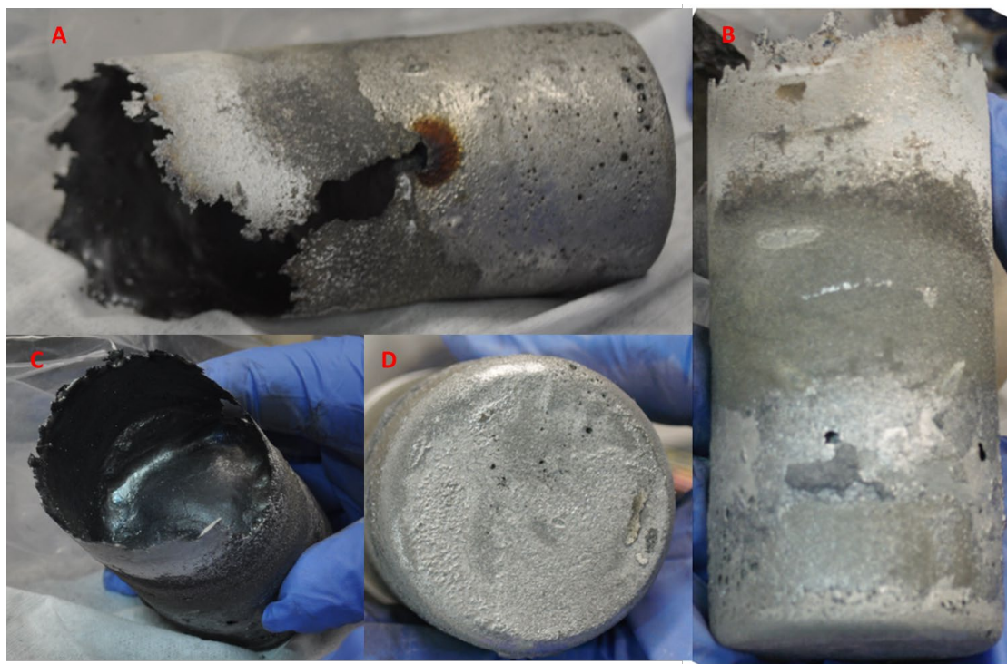
Figure 6: VC-2 billet before cleaning. A) billet side view. Just below (to the right) of where the brown halo is seen is the top of the continuous billet. Above that (to the left) of the halo is a very thin layer that was adhered to the crucible walls but not part of the continuous billet. B) The opposite side view of the billet. C) Top view of the billet which was exposed to the VIM atmosphere. The thin layer adhered to the crucible can be easily seen extending past the top of the billet. D) The bottom of the billet which was in contact with the ZrO_2 crucible
